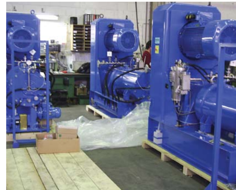
The LME Horizontal Bead Mills, with patented Dynamic Classifier System (DCCS), provide increased throughput rates with virtually no blockage.
