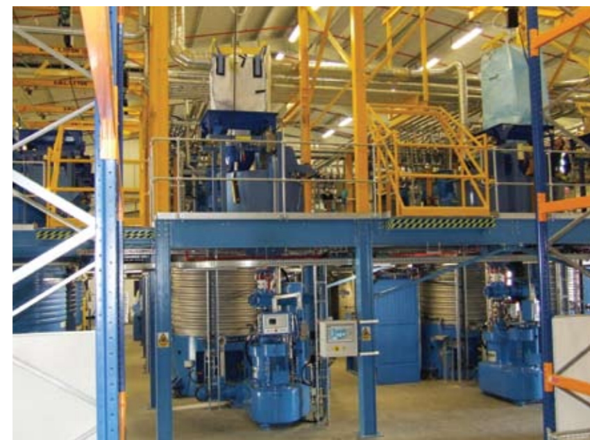
The revolutionary PSI Mixers used in the plant, with a combination of vacuum dispersing, shearing and pressure wetting resulted in high productivity, with excellent results and total reproducible quality.
